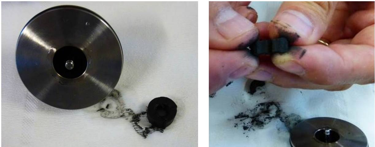
Fig 3. Broken magnet of the impeller shaft.
